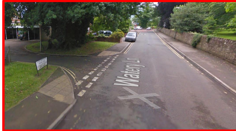
View eastwards along Watery lane showing adopted public footway to both sides of the highway, along with drop kerbs with tactile paving and double yellow lines.
